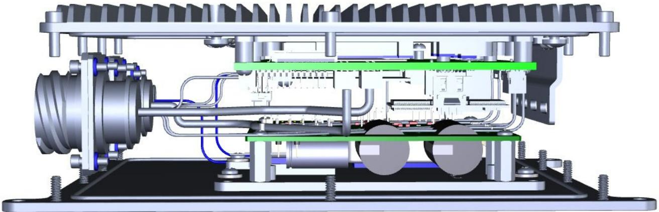
3d side view showing JMM-7500 power supply mounted to bottom cover (flat exterior surface) and VNS776KL-xGD SBC mounted to the top cover (with heat sink fins).
