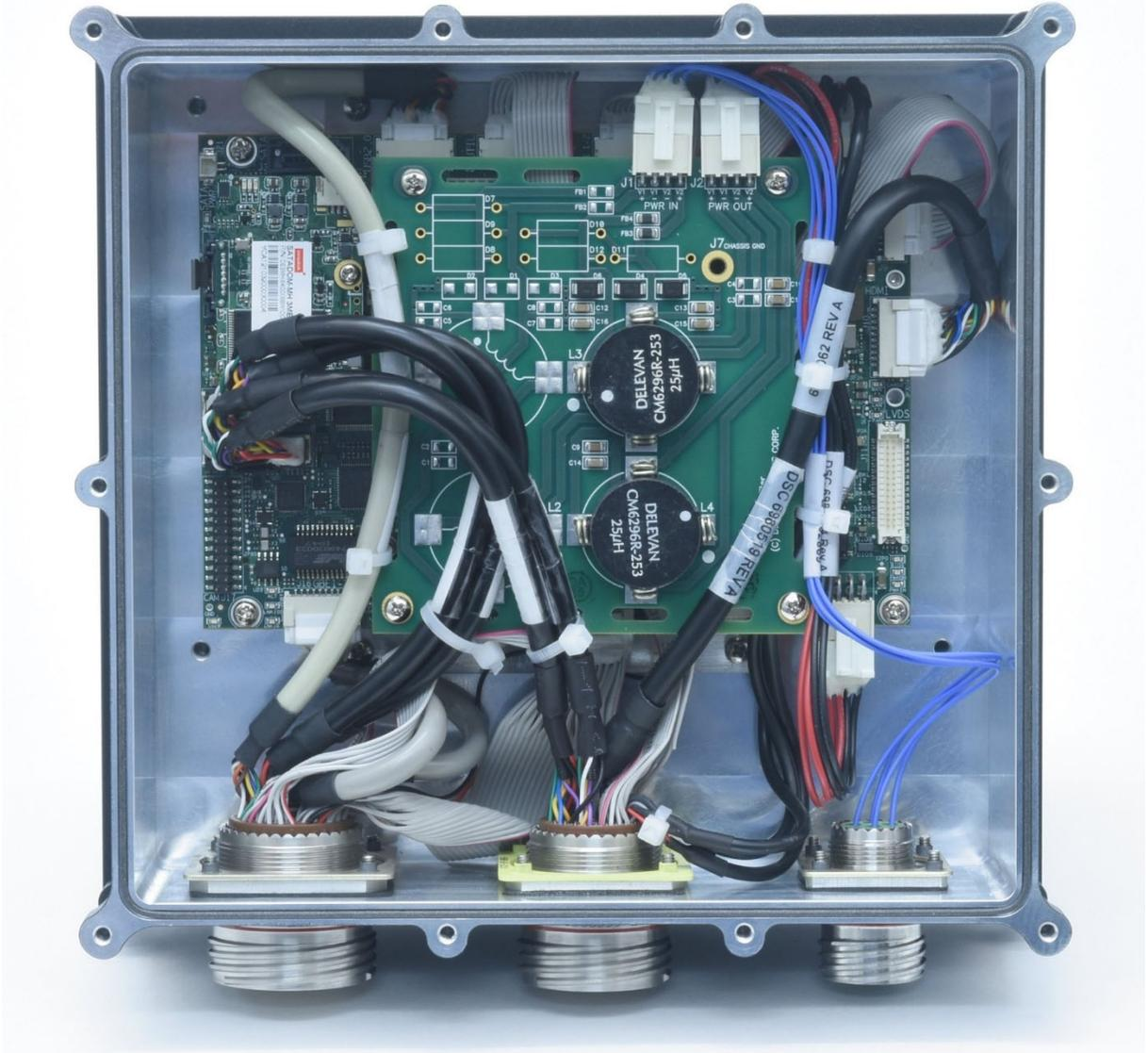
Internal view from bottom of enclosure (bottom cover and JMM-7500 power supply removed)
