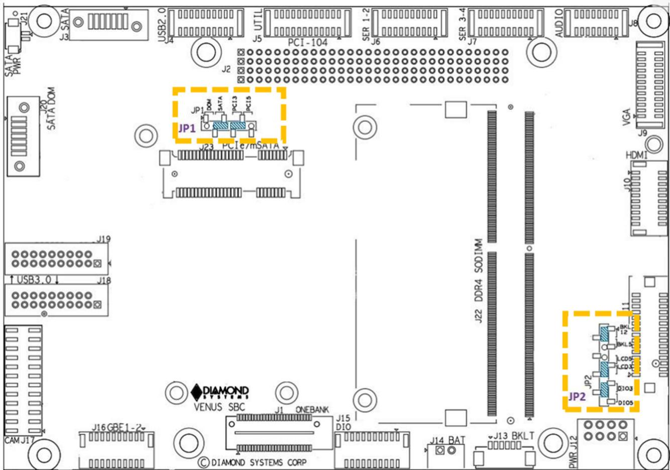
Figure 2: Jumper Blocks on Venus Carrier Board
