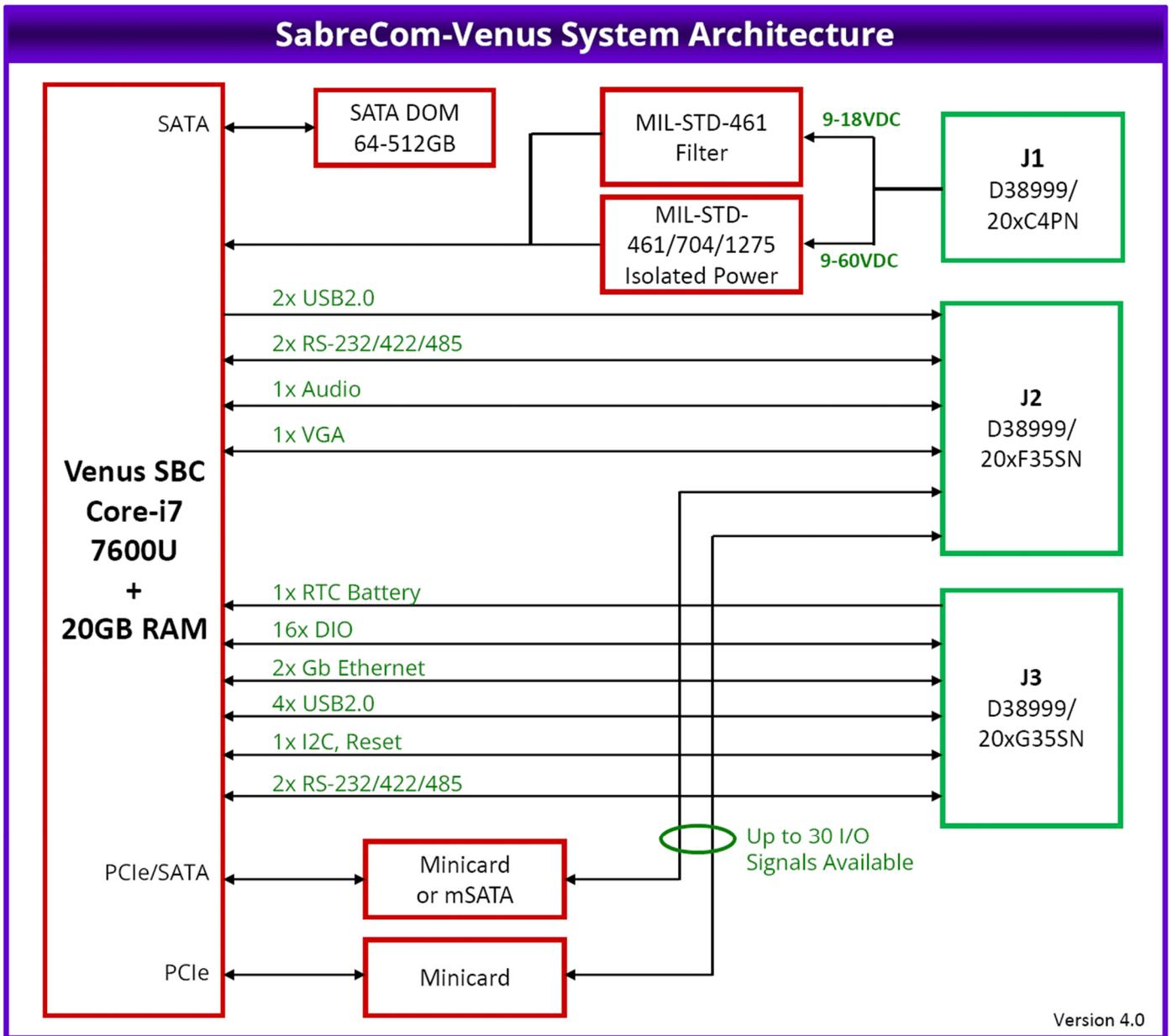
Figure 1: System Architecture of SabreCom-VNS
